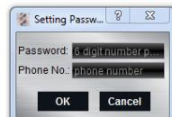
The very first time the memory function is used, it is necessary to set a 6-digit security code to save a preset. Additionally, a phone number\* shall be entered
